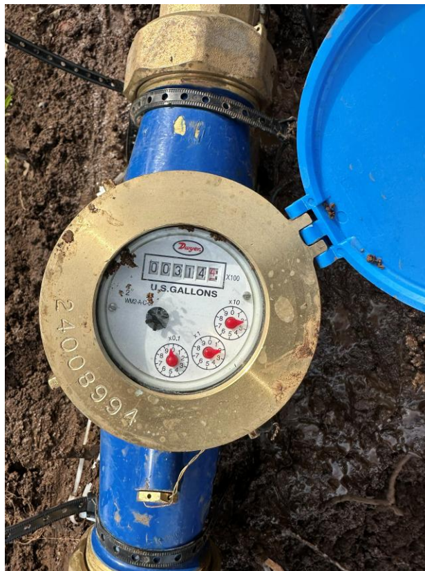
Photograph 12. Totalizer used to record volume of water injected into reverse tile drain system.
