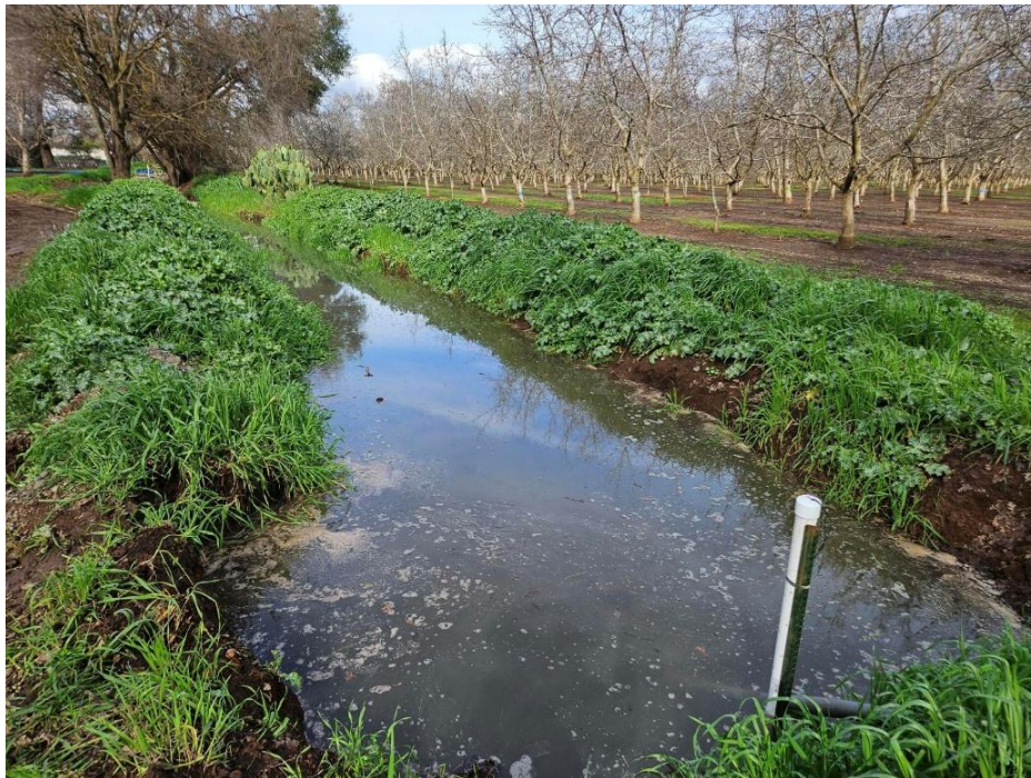
Photograph 16. Stilling well at south end (effluent) of infiltration basin.
