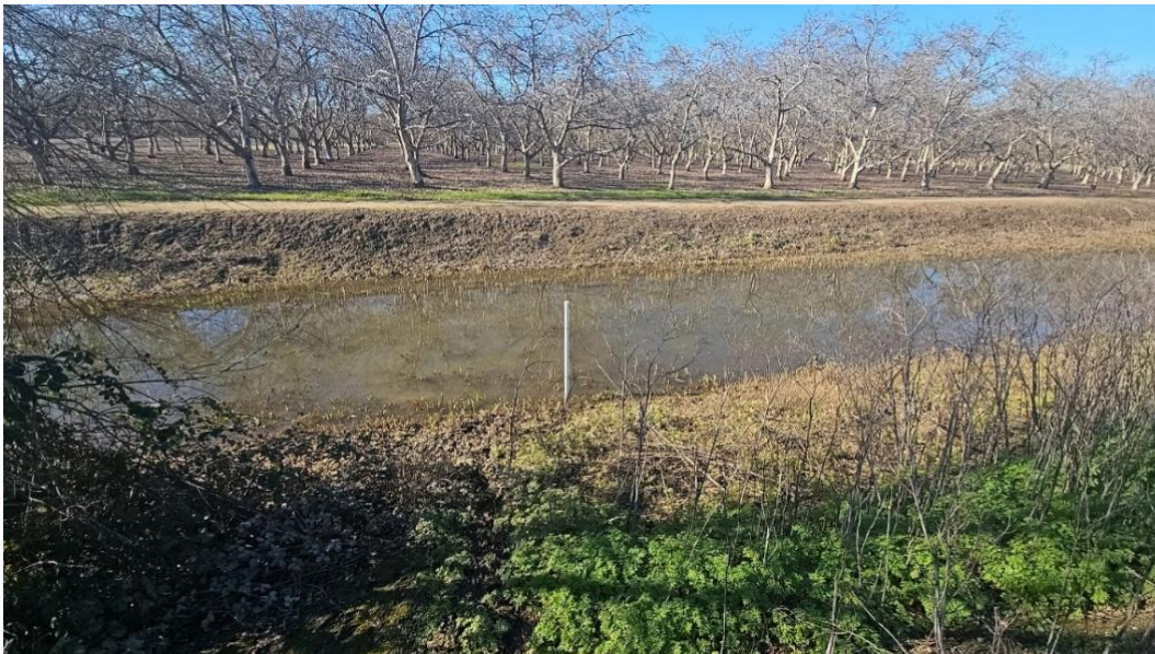
Photograph 17. Site N3 infiltration basin pilot test. White pipe is stilling well with pressure transducer inside to record changes in water levels over time.
