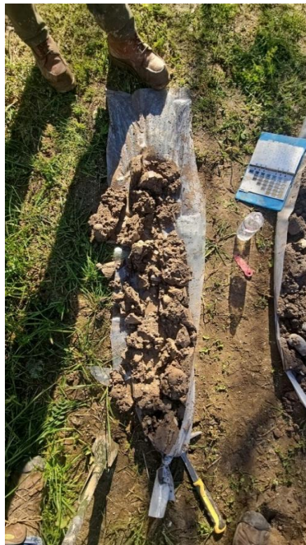
Photograph 4. Continuous core sample collected during drilling.
